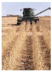
A Gleaner K2 combine, equipped with electronic weight and moisture gathering equipment, harvests a soybean plot at the Wabasso, Minn. site.
