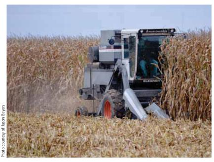
Our plot combines are modified versions of those used widely by farmers to harvest. These machines collect grain from individual plots. Grain weight and moisture is electronically measured then entered into a computer for later analysis.
